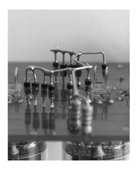
Mount the two 47K resistors in the red marked holes. Mount the 11 diodes in the green marked holes, the anode sides go into the hole. Bend all the ends that face up and connect them together. Keep it all as low as possible, so that when everything is put back together again, you don't create any shorts against the steel bottom plate. That's it folks! Enjoy!
