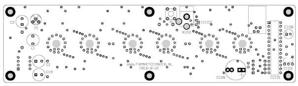
Some parts go at the bottom. Note the orientation of the 5V regulator near the DC input connector. Also take care mounting the capacitors, placing them in the right direction (polarity).
