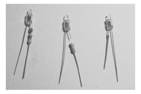
Cut away the resistor. Try to cut away the copper, leaving as much wire as possible. I often manage to bend the crimp open. Find a piece stiff wire, and make the short leg longer. Now you can feed the wires through the plastic standoff, and mount it on the PCB. Do not solder for too long, or the wire may run too hot and unsolder itself from the neon lamp. Pull the lamp gently to check if it actually is still connected inside the plastic standoff.
