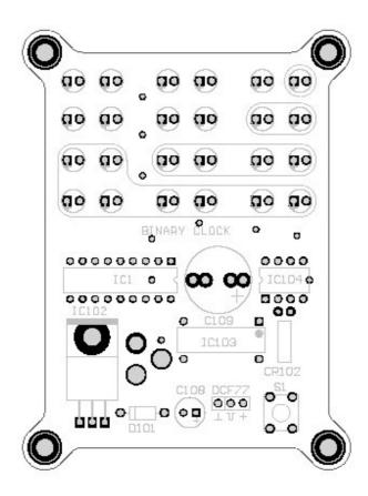
This picture shows which parts should be fitted on the top.
