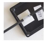
Next we need to connect the cable to the receiver. Depending on your project, you have a DCF77 or a WWVB receiver module. Put the antenna and receiver board in the box, and use some glue to keep them in place.
