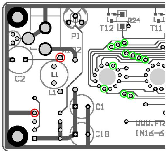
Mount the two 47K resistors in the red marked holes. Mount the 11 diodes in the green marked holes, the anode sides go into the hole. Bend all the ends that face up and connect them together. Keep it all as low as possible, so that when everything is put back together again, you don't create any shorts against the steel bottom plate. That's it folks! Enjoy!
