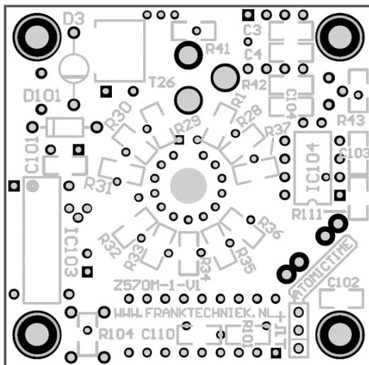
This picture shows which parts should be fitted on the top. The pushbutton can be mounted on top or bottom, whatever you like best.
